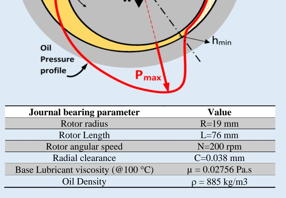
A Computational fluid dynamics (CFD) simulation approach with discrete phase modeling (DPM) of suspended nanoparticles was used.
